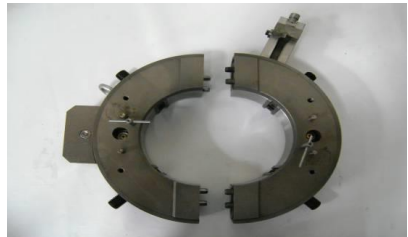
Beveling machine separated in two halves
