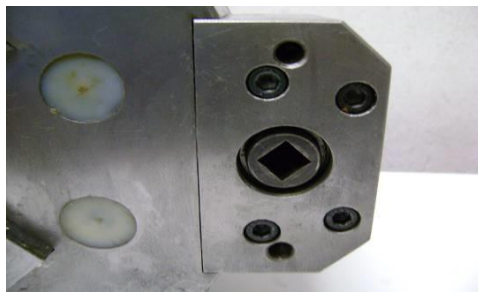
Motor flange fixation location and T wrench
