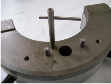
Installed lock pin
