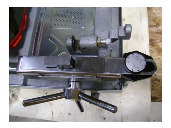
Pull and observe that there is a gear and a key under the carriage. Revome the head lock and the thread limit switch, taking special care with the springs. Loosen the brackets and remove the hose connected to the oil inlet spindle.
